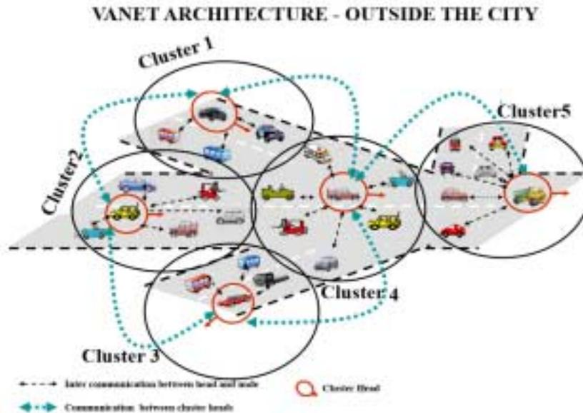
Figure1. Architecture of the VANET
